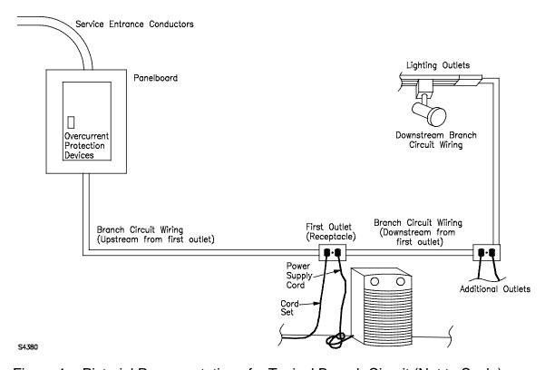
Figure 1 – Pictorial Representation of a Typical Branch Circuit (Not to Scale)
